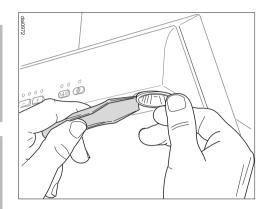
Pull the old bulb out of its socket using the enclosed lever. Replace it with a new one. Be careful not to drop the bulb on the cooktop.
